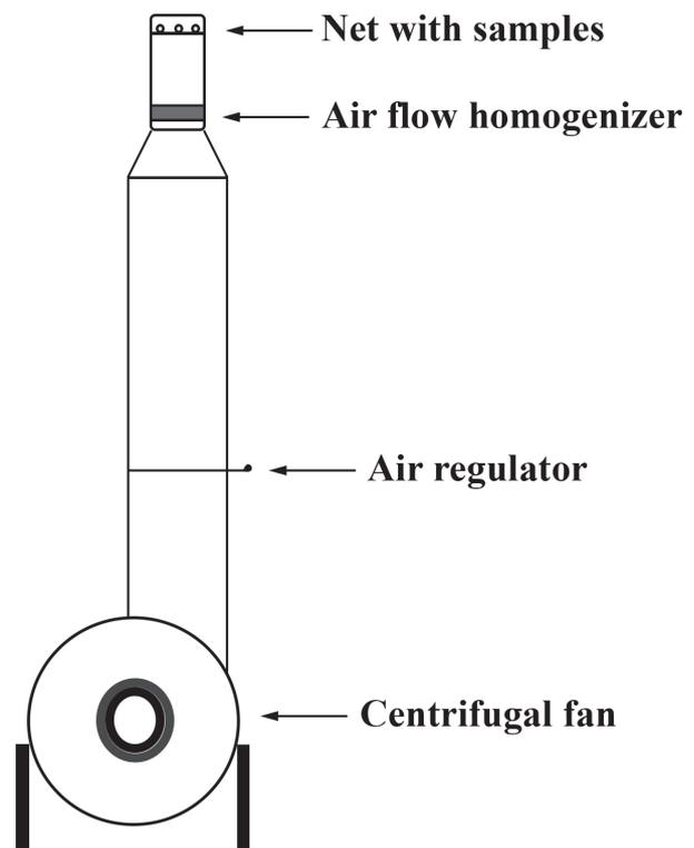
**Figure 3:** Schematic of the equipment used for measuring the terminal velocity.
