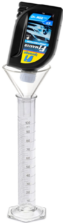
Figure 1: Illustration of the process of residual lubricant oil quantification.
