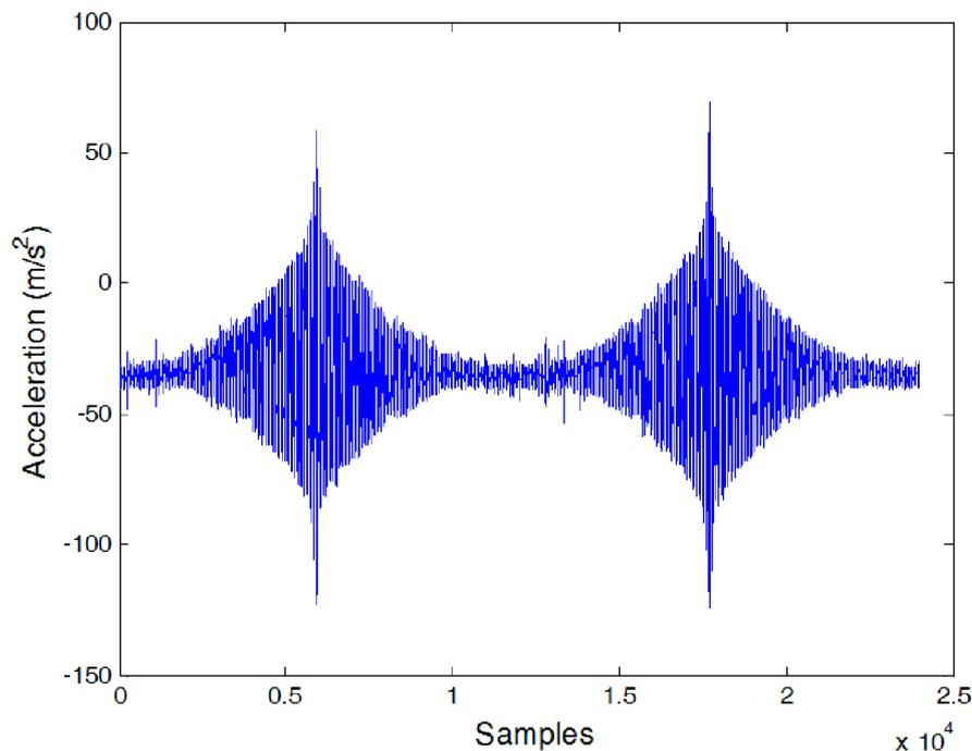
**Figure 4:** Vibration signals from the beam without failure.
