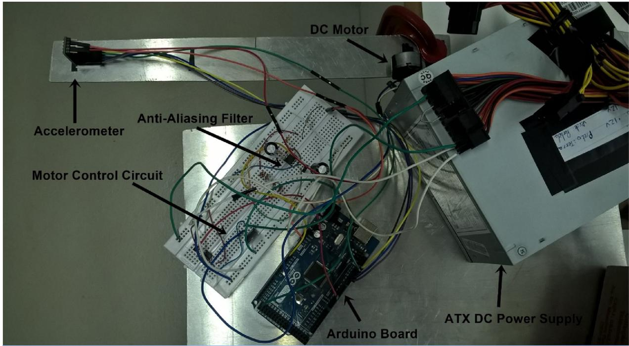
**Figure 3:** Experimental setup for signal acquisition.
