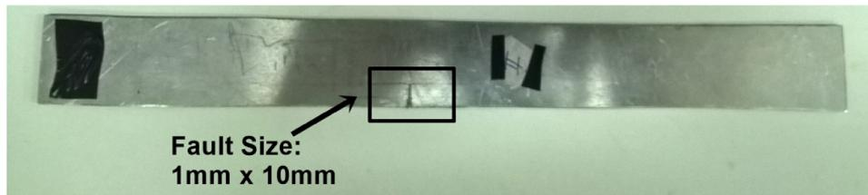
**Figure 1:** Beam used in experiment with fault.
