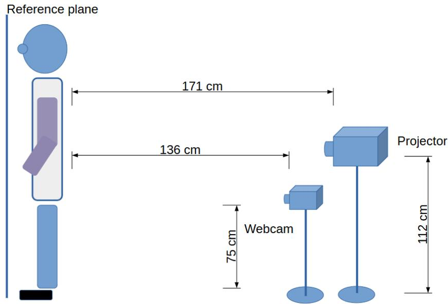
**Figure 2:** Experimental configuration with the webcam and the projector positioned in front of the object (dorsum of the volunteer).
