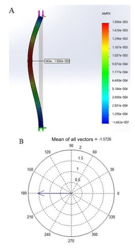
**Figure 8:** Buckling displacement using (A) FEM and (B) PIV.
