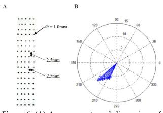
**Figure 6:** (A) Arrangements and dimensions of the marks on the sample face of lower inertia and (B) displacement vectors from the PIV technique.
