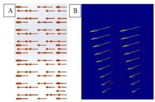
**Figure 9:** Vector images found in (A) FEM analysis and (B) PIV technique.
