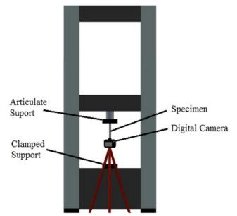
**Figure 4:** Camera position scheme in relation to the samples.
