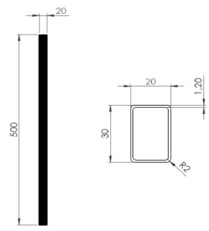
**Figure 2:** Sample details for the PIV technique evaluation.
