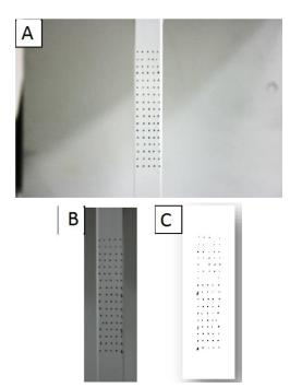
**Figure 5:** Image treatment on ImageJ software: (A) extracted image of the camera (B) Cropped Image, (C) image in RGB format 8 bit with the application of black and white threshold.
